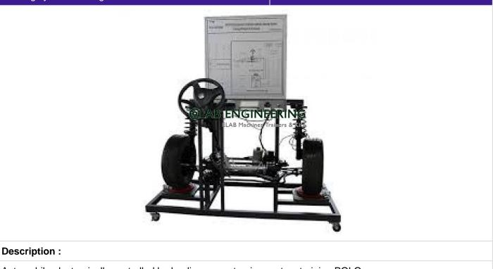
Automobile electronically controlled hydraulic power steering system training POLO
